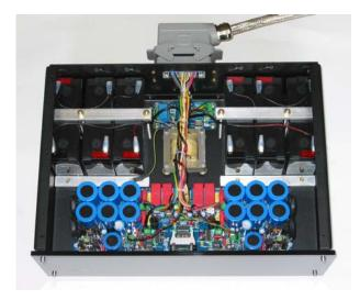
The amplifier part of the **ASR Emitters Eclusive** series has a solid transistor mounting bar made from **massive brass**.
